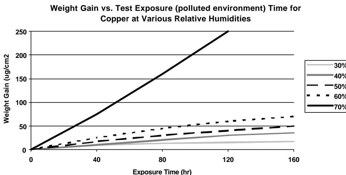
The Instrumentation Society of America information indicated corrosion could be measured at 0.01 ppm over a period of one month. This recommendation was based on sensitive instrumentation such as fine gauge computer filaments. The draft proposal which the NDEQ sent out for public input included an uncertainty factor of 2 which resulted in a standard level of 0.005 ppm.
