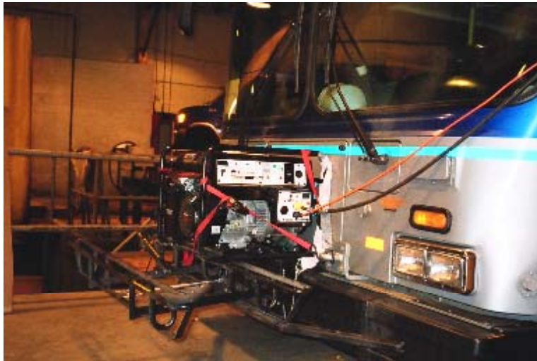
Figure 5. Generator Mounted to Front of Transit Bus
